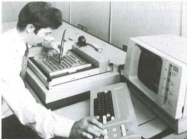
FIG. 4—Automatic fault isolation using guided-probe technique
