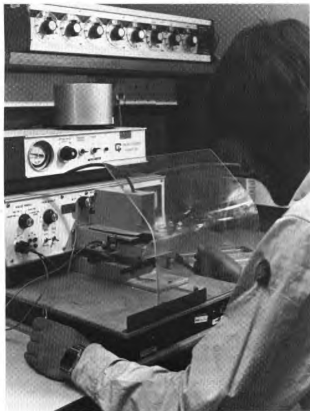
FIG. 5—Adjusting resistors by air-abrasive trimming
