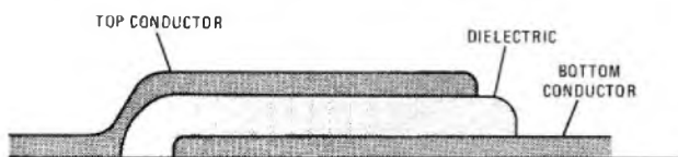
FIG. 3—Section through a thick-film capacitor
