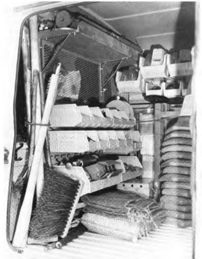
FIG. 12—Layout of tools and stores for faultsman-jointer's vehicle
