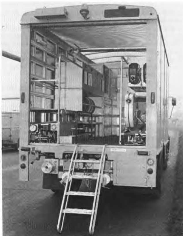
Note: This unit is operated by 2 men, and incorporates a rod-pushing machine and a cabling winch
