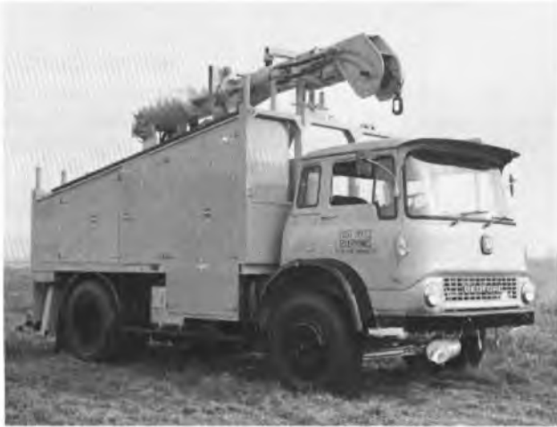
Note: This unit is operated by 2 men. It has a power auger for hole boring, and a crane for lowering in the poles
