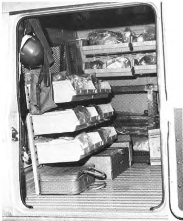
FIG. 11—Layout of tools and stores for installer's vehicle
