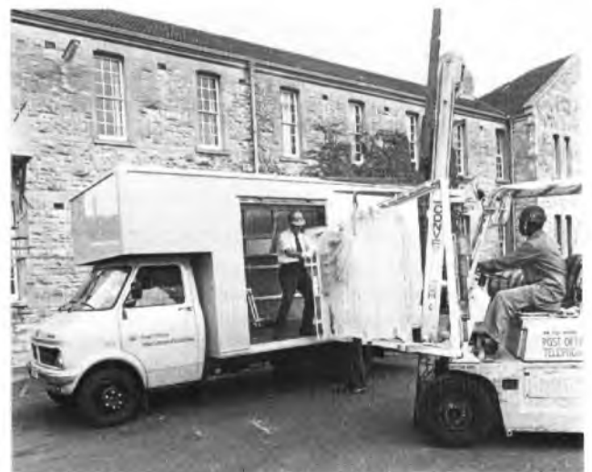
FIG. 6—A 30 cwt closed stores-carrying vehicle
