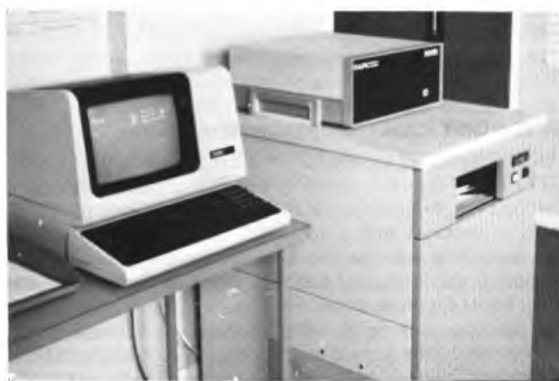
FIG. 2—Facsimile printer and printer-operator's terminal
