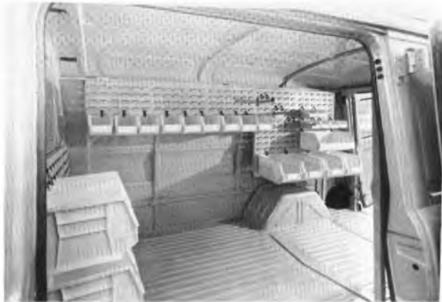
FIG. 10—A 15 cwt utility vehicle fitted with louvred panelling
