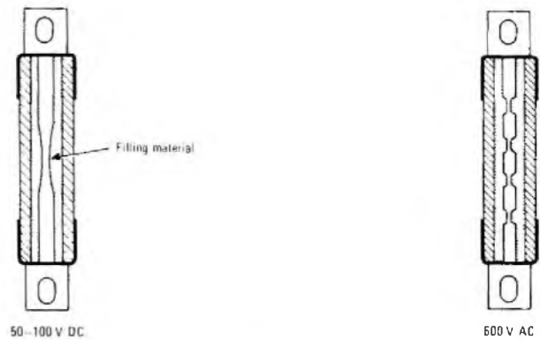
FIG. 4—Typical fuse elements
