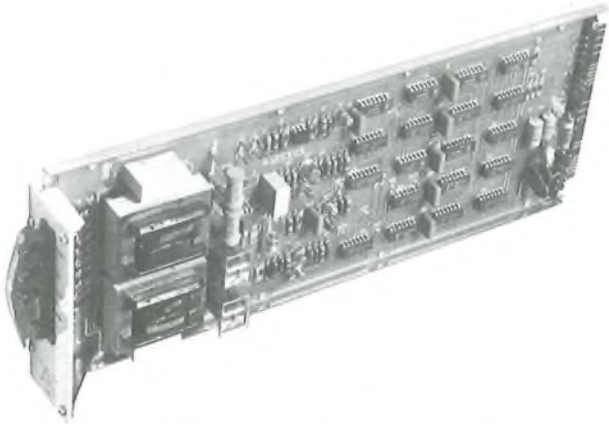
FIG. 31—Incoming PCM signalling unit (Photograph by courtesy of GEC Telecommunications Ltd.)
