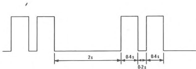
FIG. 4—Cadence of British Post Office ringing tone
