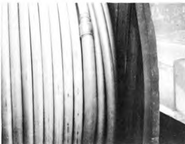
FIG. 2—Diversion cable on drum, showing weld at one end of the unidiameter joint
