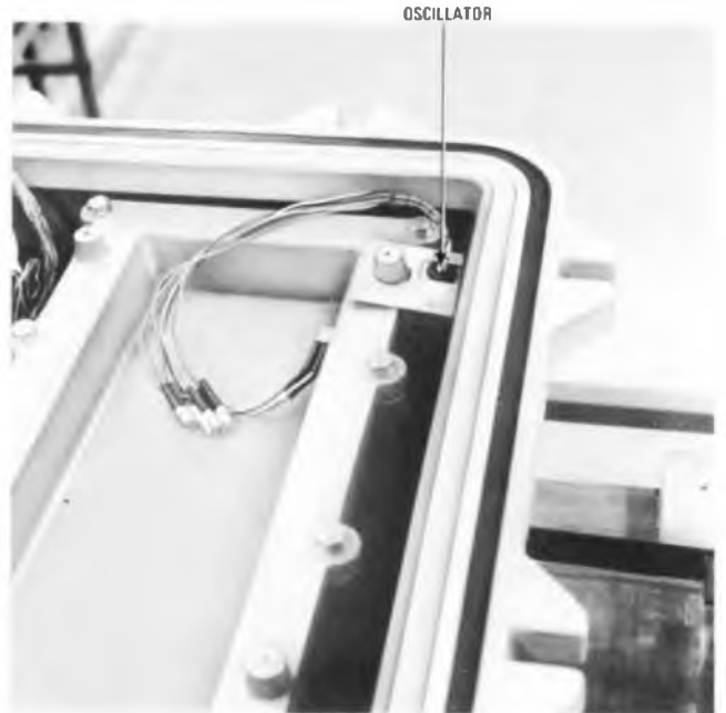
FIG. 3—Contactor oscillator in situ in the 60 MHz repeater case
