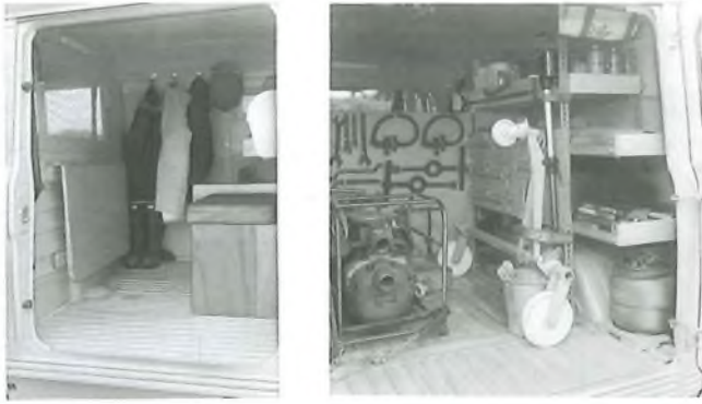
The personnel compartment (left) viewed through the side door, and the equipment compartment (right) viewed through the rear doors
