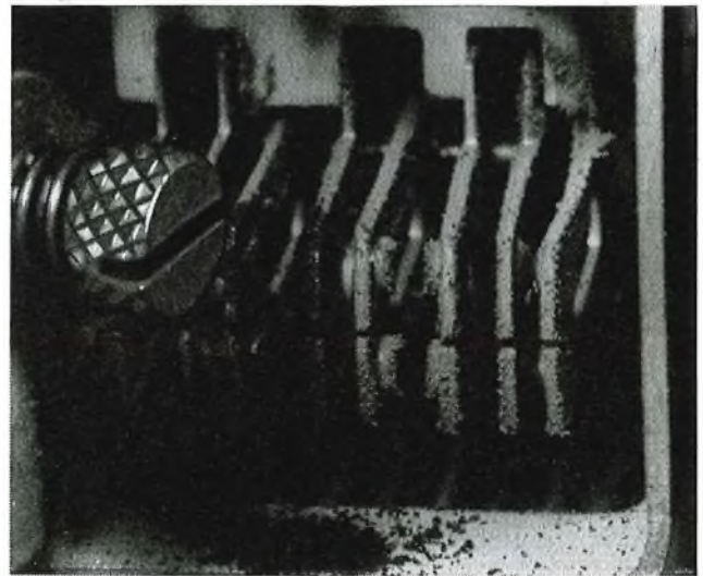
FIG. 25—Carbon particles and dust from arcing contacts
