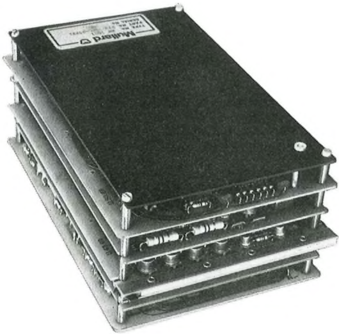
FIG. 3—The 8,192-bit ferrite core-store
