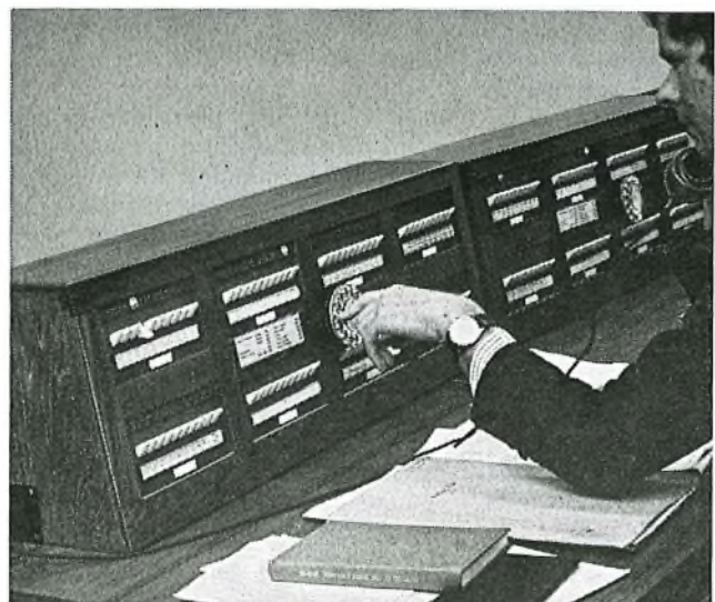
FIG. 1—Ten-line key-and-lamp units installed in a console
