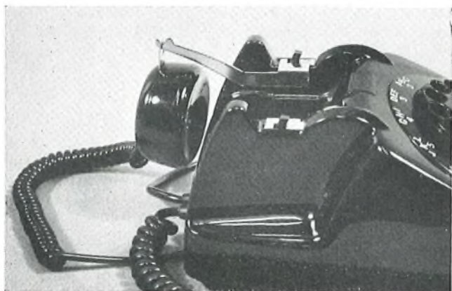
FIG. 1—WATCH RECEIVER AND BRACKET ON 700-TYPE TELEPHONE
