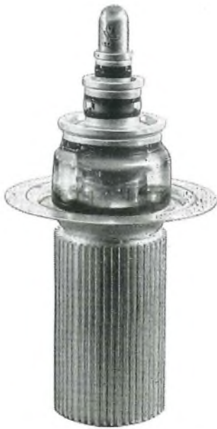
FIG. 1—CHANNELLED-ANODE TYPE OF VAPOUR-COOLED VALVE
