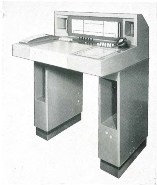
FIG. 3—S.T.C. NO. 4 CORDLESS SWITCHBOARD
