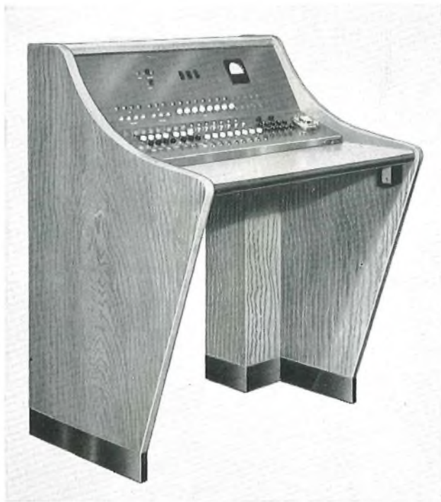
FIG. 4—E.T. NO. 4 CORDLESS SWITCHBOARD
