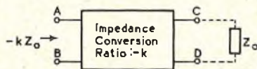
FIG. 1.—COMBINATION OF A NEGATIVE IMPEDANCE CONVERTER (ABCD) AND A PASSIVE IMPEDANCE ( Z_0 ) TO GIVE NEGATIVE IMPEDANCE.
