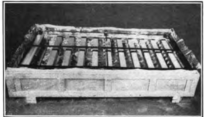
FIG. 3.—APPARATUS RACK IN CASE, SHOWING PACKING IRONS AND WATERPROOF ADHESIVE TAPES.
