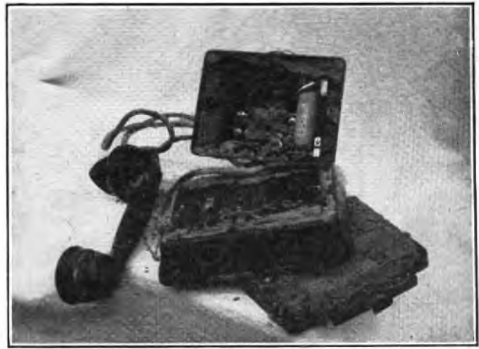
SUBSCRIBER'S INSTRUMENT AFTER PENETRATION BY SAND.
