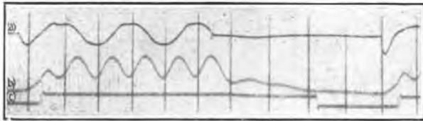
(a) Received 50 c/s A.C. Line Current. (b) Rectified Pulse Through Relay LS. (c) Output from Relay LS.
