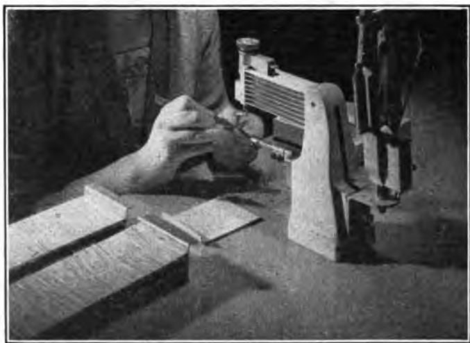
FIG. 6.—WELDING WIRES OF 1A THERMISTOR TO A CUNIFE HAIRPIN.
