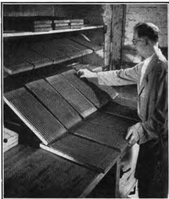
FIG. 2.—TRAYS OF BRIMISTOR MATERIAL AFTER CURING.
