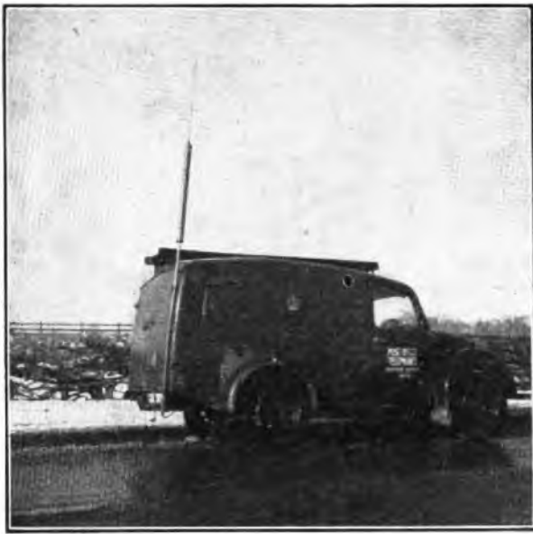
RADIO CONTROL VAN FITTED WITH V.H.F. TRANSCEIVER.
