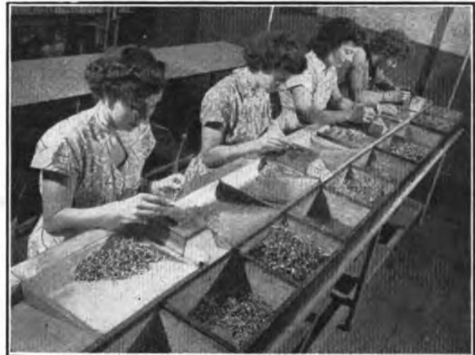
FIG. 4.—SOLDERING WIRES TO BRIMISTORS.
