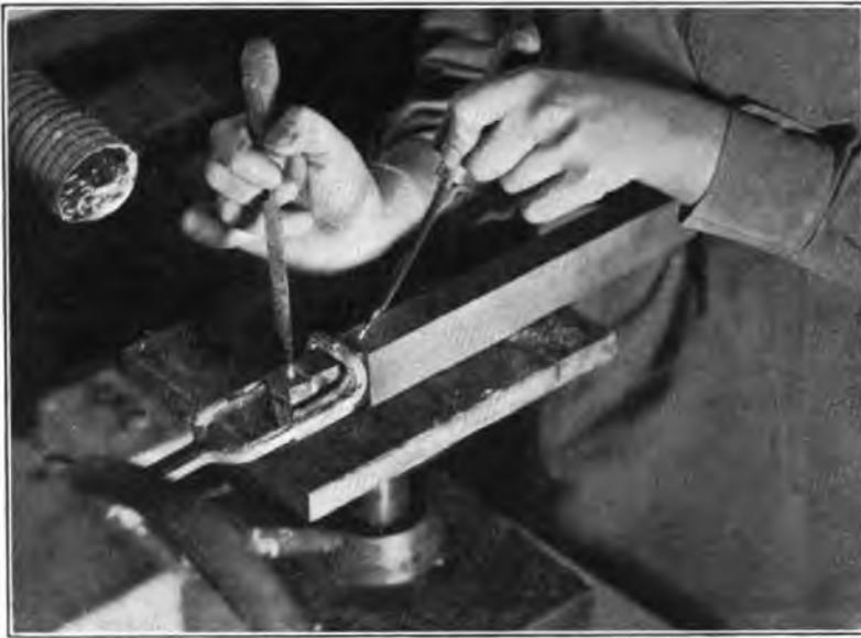
FIG. 2.—HIGH FREQUENCY INDUCTION HEATING FOR BRAZING.
