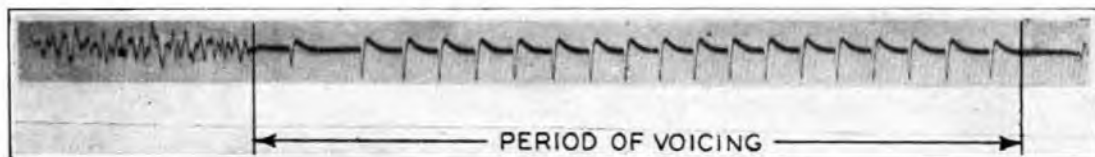
FIG. 10.—OUTPUT OF SWITCHING CIRCUIT FOR DURATION OF A VOICED SOUND.
