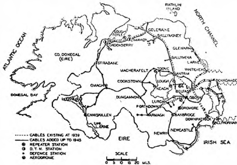
FIG. 1.—MAIN UNDERGROUND CABLE NETWORK.
