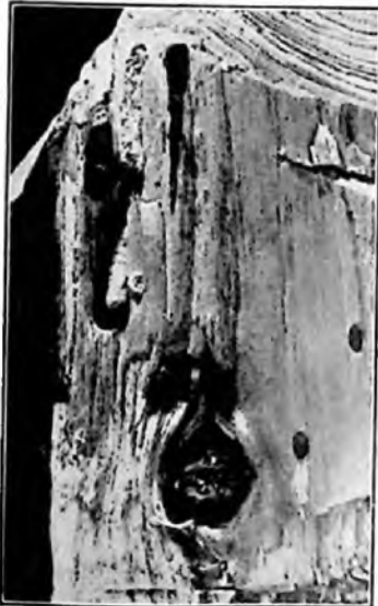
FIG. 1.—EFFECT OF LARVA ON TIMBER.
