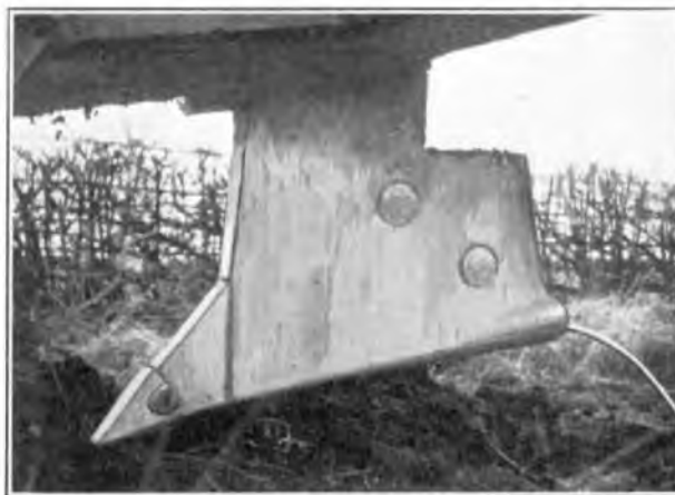
FIG. 5.—RIPPER BLADE WITH CABLE-LAYING MODIFICATION.
