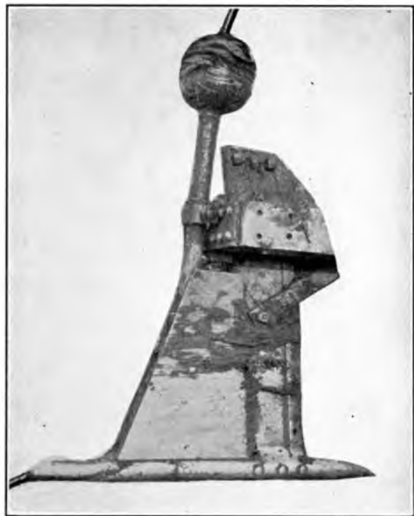
FIG. 1.—MOLEDRAINER MODIFIED FOR CABLING WORK.
