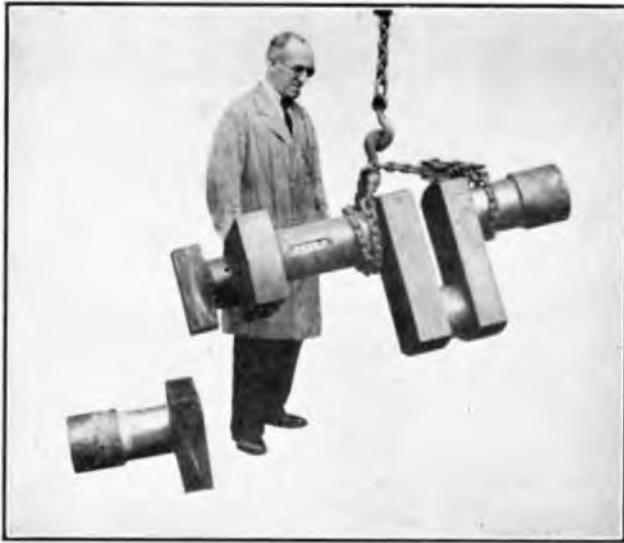
FIG. 2.—REPAIR OF 1\frac{1}{2} TON LOCOMOTIVE CRANKSHAFT
