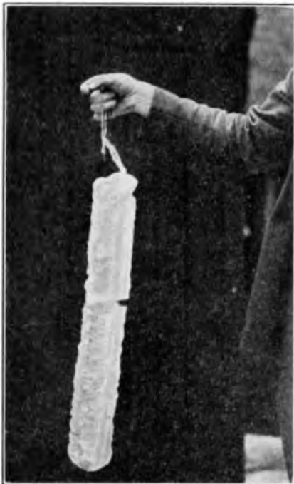
FIG. 1.—A TYPICAL ICE-COATED WIRE, WORCESTER.
