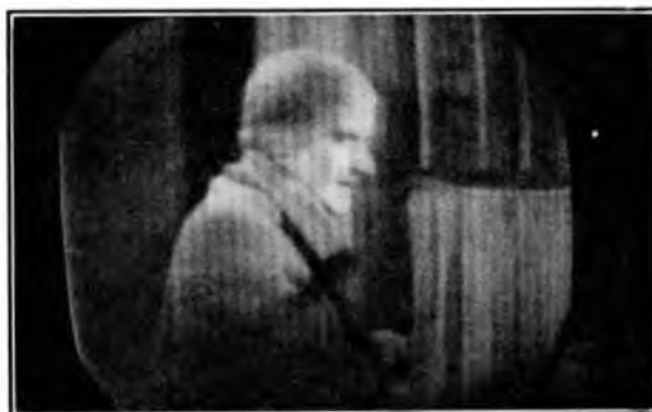
(f) Single-frequency noise, 500 kc/s approximately, mesh pattern.
