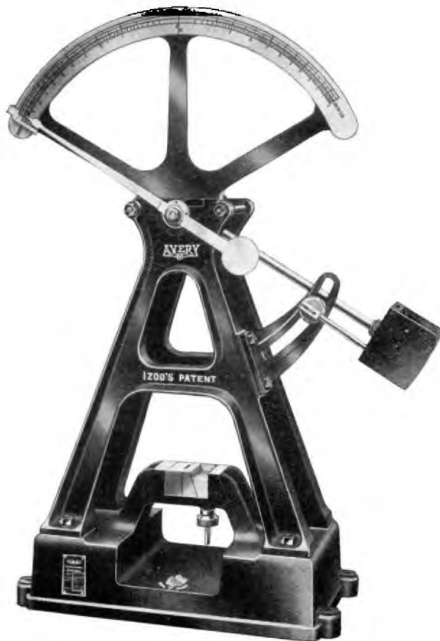
FIG. 6.—SPECIAL MACHINE FOR TESTING BAKELITE, PORCELAIN, OR GLASS.
