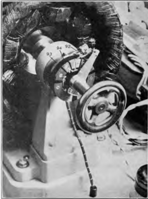
FIG. 13.—MOTOR AND DISTRIBUTOR (CORRECTING) EQUIPMENT.
