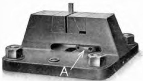
FIG. 2.—VICE FOR GRIPPING SPECIMEN UNDER TEST.
