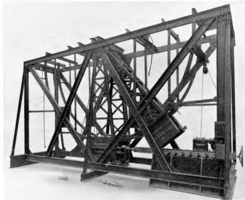
FIG. 7.—A LARGE IMPACT TESTING MACHINE FOR TESTING RAILWAY COUPLINGS AND DRAWBARS.
