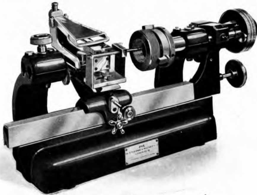
FIG. 11.—TESTING PITCH OF SCREW RING GAUGE.
