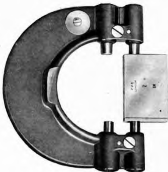
FIG. 5.—SETTING ADJUSTABLE LIMIT GAUGE WITH SLIPS.
