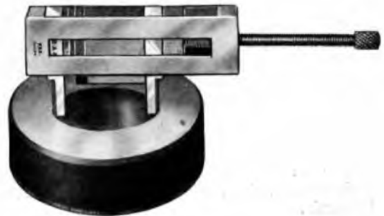
FIG. 3.—TESTING SIZE OF RING GAUGE WITH SLIPS AND JAWS.
