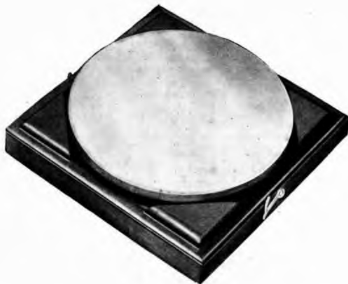
FIG. 7.—TOOLMAKER'S FLAT IN STEEL, HARDENED, GROUND AND LAPPED.
