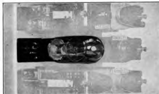
Illustration showing small size of Ballast Resistance and how it mounts in the space of a relay.
