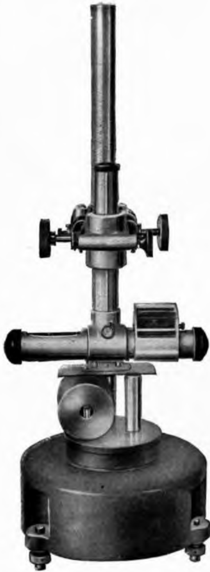
FIG. 8.—BENCH TYPE GENERATOR COMPARATOR COMPARING CYLINDER AGAINST LENGTH STANDARD.
