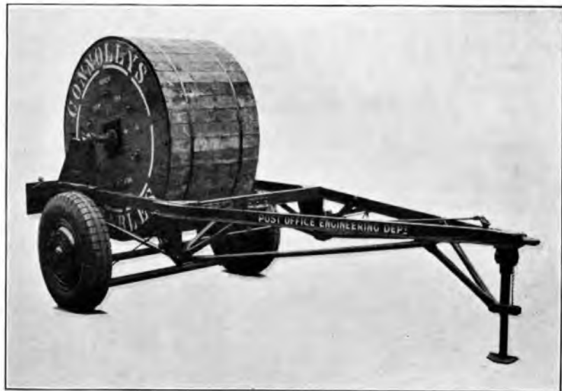
FIG. 1.—TRAILER EQUIPPED WITH SADDLES FOR CARRYING CABLE DRUMS.
