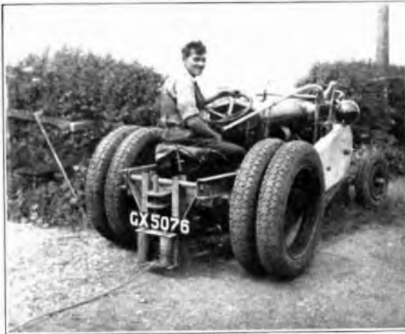
Fig. 2.—Rear view, showing steel Hawsers and Guide Rollers.
