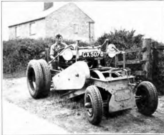
Fig. 1.—Front view of Fordson-Automower Tractor and winch, showing winding drum and one of the anchors.
