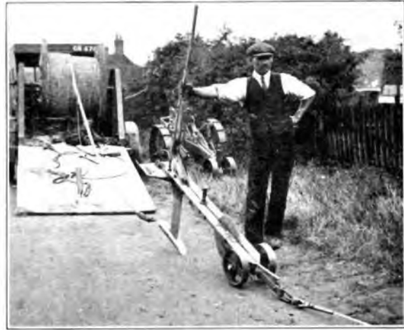
Fig. 10.—“Little Wonder” Mole Drainer (with special leading wheels and modified mole), used on narrow margins.
