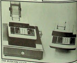
THE BUSICOM 122 CD calculator can be used on its own (right) or will automatic cash till (left). The cash draw opens automatically when the and grand total keys are pressed and a security bell rings. Retailing at 1817 AT, the machine is available from Broughton & Co, 6 Priory Road. Children & Co, 6 Priory Road.
