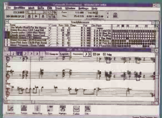
Main control screen showing Track/Measure window and Staff window with multiple staves
