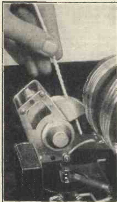
A pipe cleaner will remove dust from between the vanes of a variable condenser. Many of the crackling noises which are heard when a short-wave set is tuned are due to the presence of dust.
