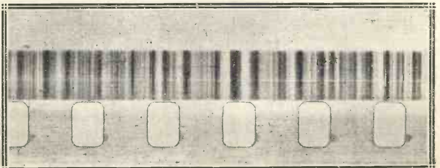
This section of a 35-mm. film depicts an actual photographic record of a group of waves obtained by means of a cathode-ray oscillograph.
