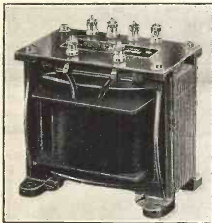
An output transformer like this costs money, and while it will match certain loudspeakers to a particular power valve, the absence of a standardised loudspeaker impedance may render the transformer useless if other speakers are bought.
