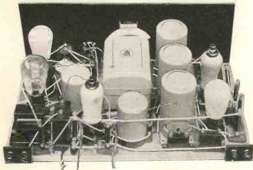
All interaction of high-frequency fields is rendered impossible by the metal screening. Gang condenser, coils, intermediate transformers and H.F. choke all have cans, and the baseboard is covered with copper foil in addition.
