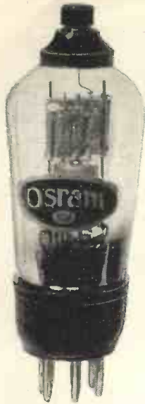
The Osram double-diode triode, M.H.D.4, carries out rectification, L.F. amplification and automatic volume control at one and the same time.
