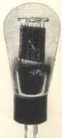
The latest Mullard super-power 4-volt A.C. valve, the D.O.26, which gives about 7.5 watts undistorted output.
