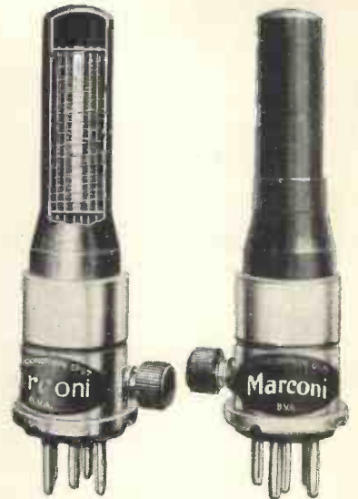
The Catkin M.P.T.4, showing the enamelled anode, and also this electrode cut away to reveal the inner structure.
