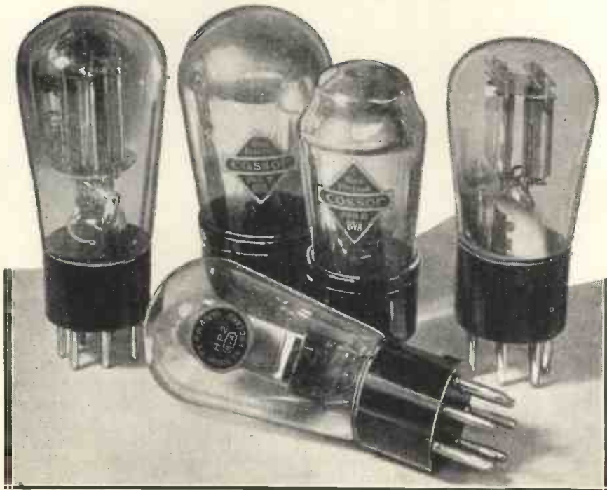
A group of positive drive output valves. They are Mazda P.D.220, Cossor 240B and 220B, Mullard P.M.2B., and Ferranti H.P.2. Note the special non-microphonic bulb of the 220B.
