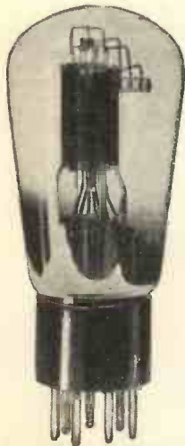
The 7-pin indirectly-heated cathode power pentode, Pen.4.V.A.
