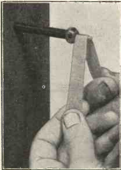
When the volume falls off don't forget to examine the aerial system. If the lead-in insulator connection is dirty, clean it up with a strip of emery cloth.
