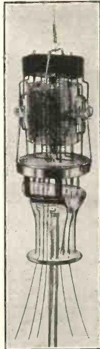
The internal details of an up-to-date power pentode—the Pen.4V.A. Note the 7 pins.
