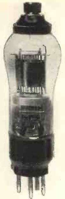
The V.P.T.4 is a multi-mu version of the S.P.T.4. It comes from the Ferranti factory.
