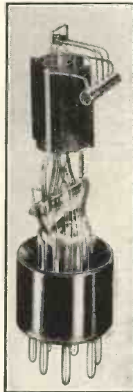
The internal details of an up-to-date power pentode—the Pen.4V.A. Note the 7 pins.
