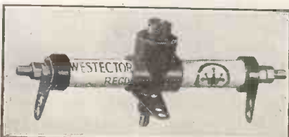
For full-wave detectors. This is one version of the now well-known Westector made by the Westinghouse Company.
