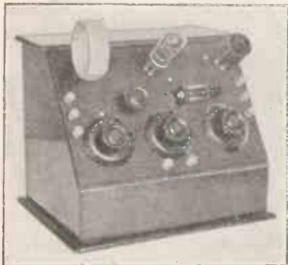
The first home constructors mounted all their components on an ebonite panel which formed the lid of a box dignified by the name of "cabinet."
