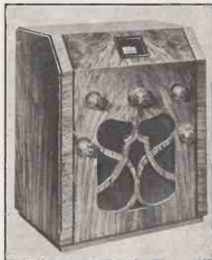
The slope of the top front part of this Telsen receiver, on which the escutcheon is mounted, makes the dial readings particularly convenient to see.
