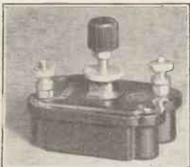
The preset condenser is a small component, but it makes a big difference to selectivity when joined in series with the aerial lead.
