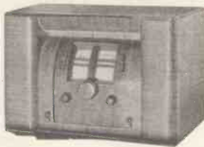
This new Reico set is arranged to switch to short, medium, or long wavelengths, and is evidence of Germany's growing interest in the short waves.
