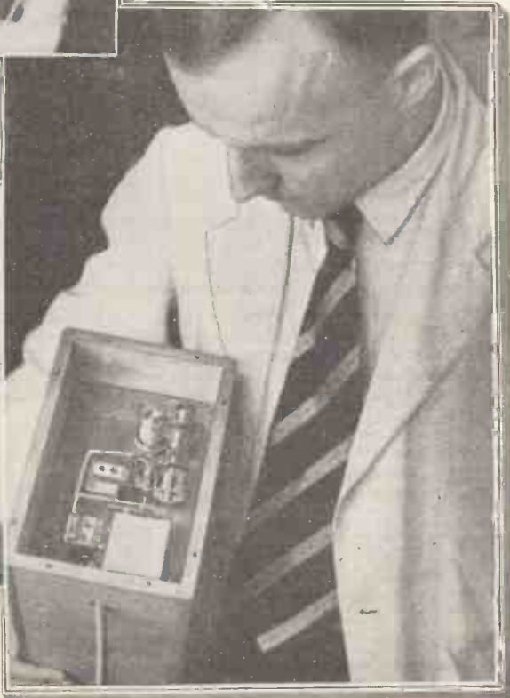
A close-up of the apparatus which, using no microphone, is more stable than an acoustic system.
