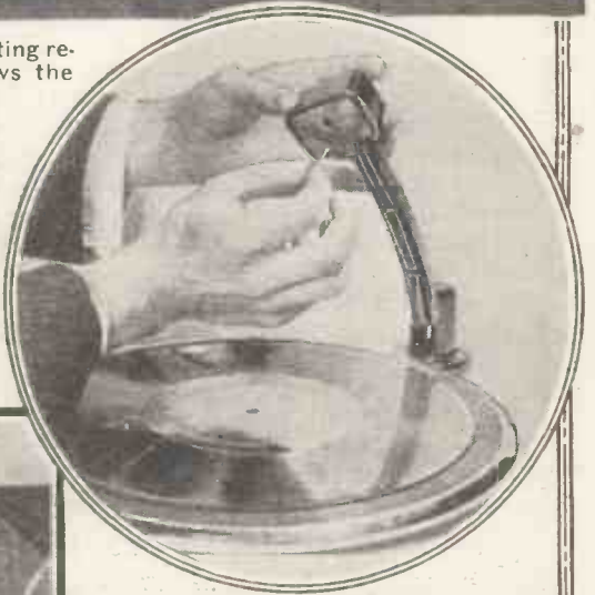
The Philips' pick-up (above) has a useful vertical lift which increases the ease with which the needle can be inserted.
