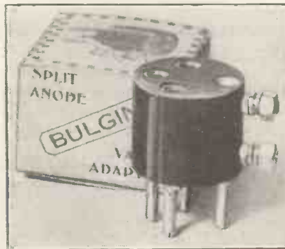
By inserting this adaptor plug between the valve and its holder, and connecting a meter across the terminals, the current of each individual valve may be tested.
