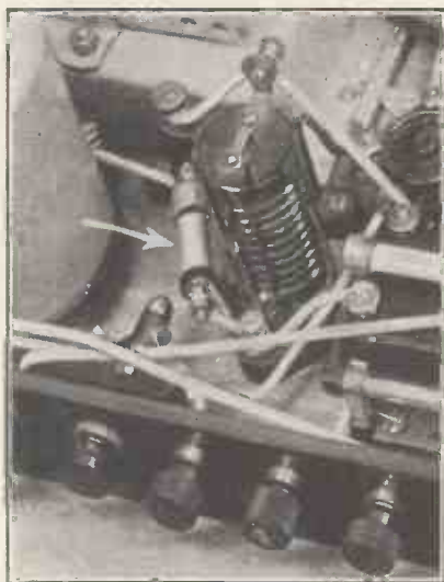
The Westector—to which the arrow points—is a small edition of the Westinghouse metal mains rectifier. In size it is comparable with a grid leak.
