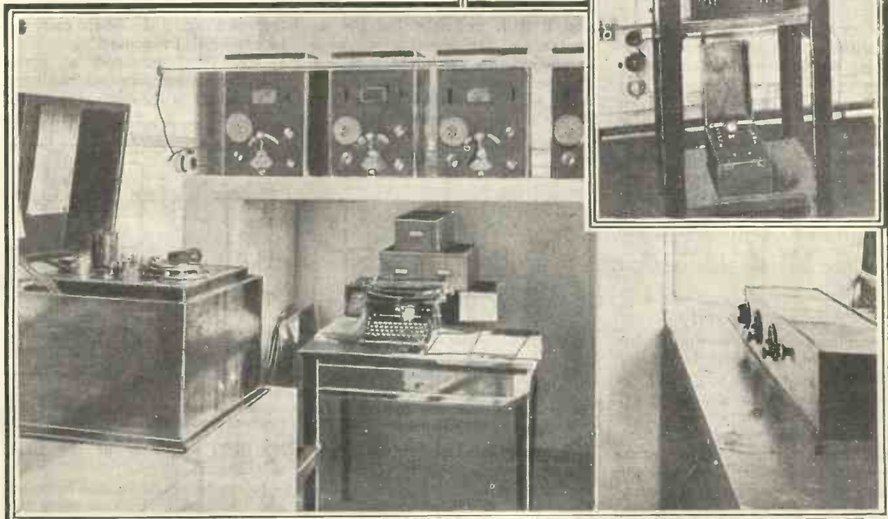
A corner of the listening room where the main wavemeters are housed. Four Sullivan type meters for different ranges are visible ranged along the shelf, and to the left is the Brussels wavemeter. This is a sub-standard of one kept at the international wavelength measuring station at Brussels.
