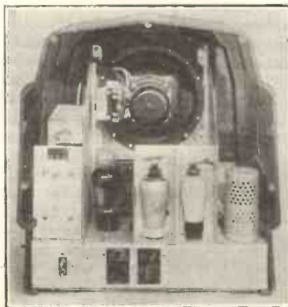
Note how the valves are easily accessible and how complete screening is given to the various stages to ensure stability.
