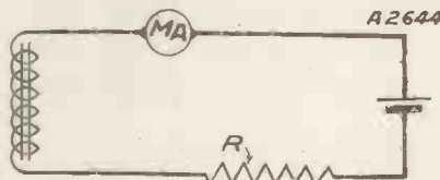
This shows how a grid-bias battery and a resistance can be connected to a milliammeter for measuring the D.C. resistance of a choke or transformer coil.
