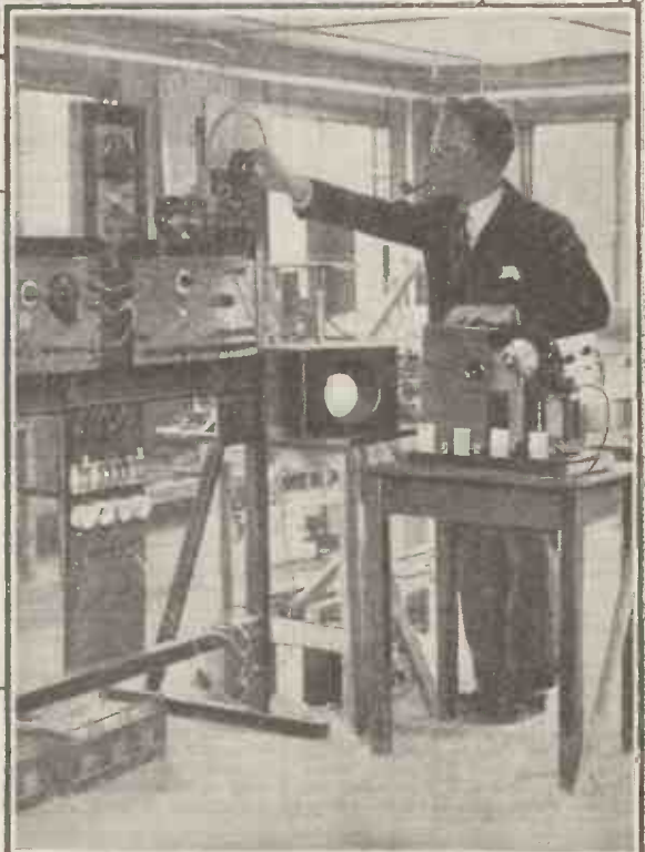
On the left : Mr. Brown, who is spending his time operating a 3-kilowatt Tulse transmitter, which is used at Simavik to transmit to Tromso. And on your right : Mr. Geoffrey Builder (Professor Appleton's second-in-command) with his super-heterodyne receiver fitted with cathode-ray oscillograph and recording camera for photographing echo.
