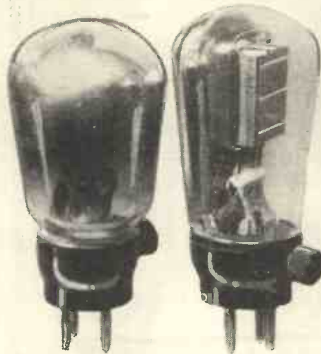
Here are two more high-efficiency battery pentodes. The Mazda Pen.220A. on the left, and the Cossor 230P.T.
