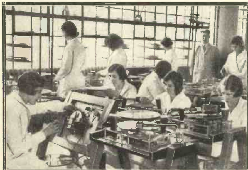
A new simplified method of constructing the H.M.V. automatic record-changing mechanism has recently been introduced at one of the factories at Hayes. The chassis are mounted in jigs which can be tilted at any angle to facilitate adjustments, while overhead conveyors do a great deal to speed up production.
