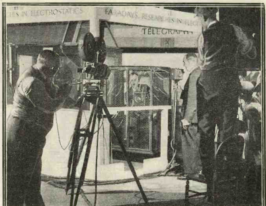
Making a sound film of one of Faraday's famous experiments; that of a man sitting inside a metal cage charged with a pressure of 250,000 volts.
