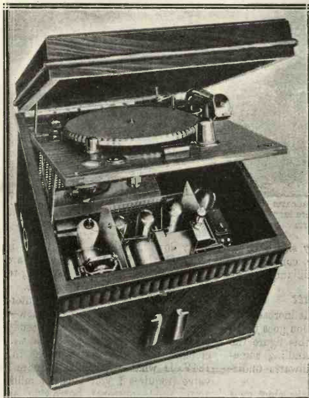
An example of German radio-gram construction. Note the compact stowing away of the multitudinous parts.
