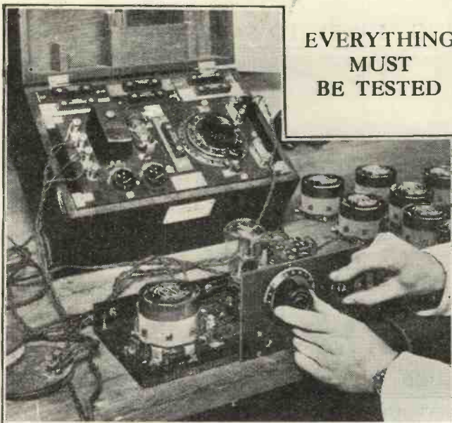
Probably the only way in which the manufacturer scores over the home constructor is in that he can afford expensive testing apparatus so that no faulty components need find their way into completed receivers. Here we see coils being tested in the R.I. factory.
