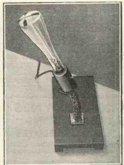
When this cathode ray tube swings to and fro the light-spot at the free end of the tube moves under the influence of the earth's magnetism.
