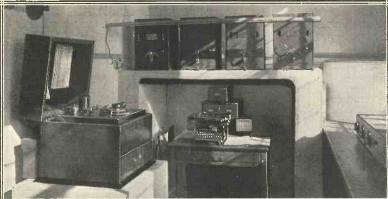
On the left of this photograph you can see the Brussels wavemeter, which is used to check-up the wave-lengths of the transmitting stations. This meter is, in turn, checked up by tuning-fork multi-vibrators.
