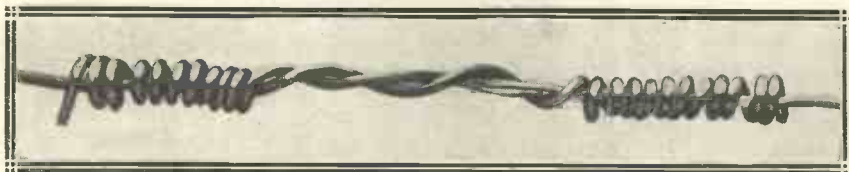
This is the tight-grip joint referred to on this page.
