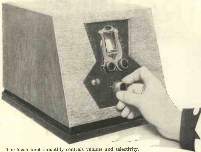
The lower knob smoothly controls volume and selectivity.
