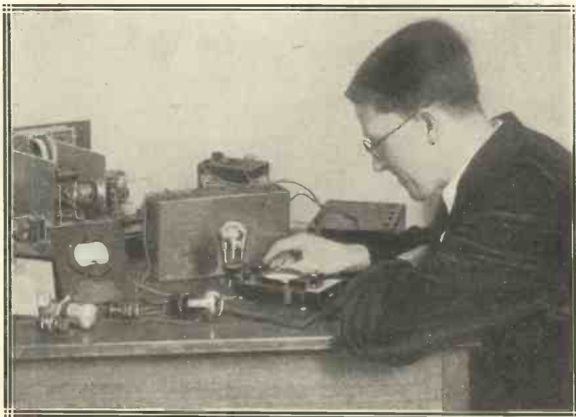
A member of the Research Department testing a new valve. Careful measurements are taken before the valve is tried out in a set, under practical conditions.
