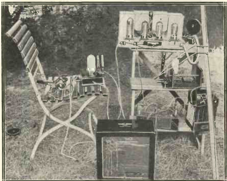
A short-wave receiver used in some open-country receiving tests on which Von Ardenne's scheme was based.
