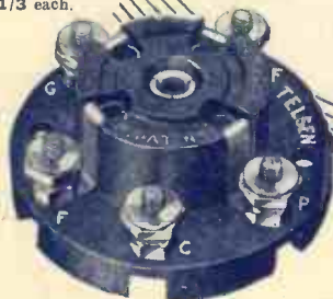
TELSEN VALVE HOLDERS. Pro. Pat. No. 20286/30. An entirely new design in Valve Holders, embodying patent metal spring contacts, which are designed to provide the most efficient contact with the valve legs, whether split or non-split. Low-capacity, self-locating, supplied with patent soldering tags and hexagon terminal nuts.
