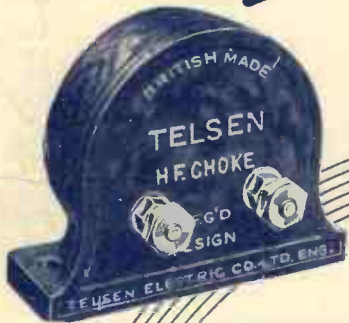
TELSEN H.F. CHOKES. Designed to cover the whole wave-band range from 18 to 4,000 metres, extremely low self-capacity, shrouded in genuine Bakelite. Inductance 150,000 microhenries. Resistance 400 ohms. Price 2/6 each.
