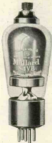
This is the most recent addition to the ranks of S.G. A.C. valves. It has an impedance of only 257,000 ohms and a magnification factor of 900.
