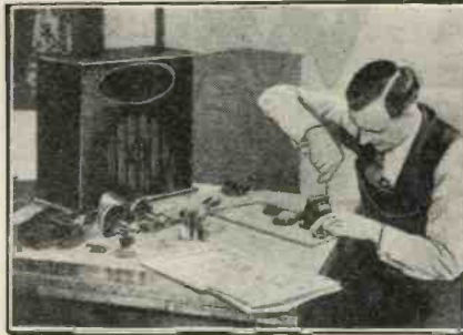
You commence the construction of the Brown S.G. Three by tackling the mounting of the components on the baseboard.
