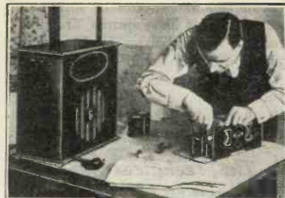
When the panel components are in position and wired up the set is ready for test, and the whole job need not occupy more than three or four hours.
