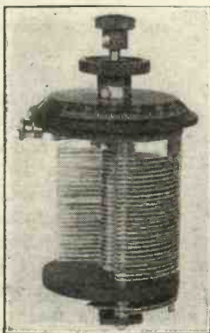
Left and right you see two variable condensers dating back about five years. With their ebonite end plates and straight-line-capacity vanes they look very crude as compared with the Polar "Tub," a very recent shielded gang assembly due to Messrs. Wingrove and Rogers.
