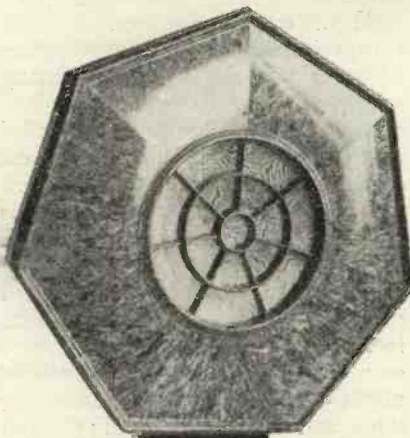
The moving-coil principle in loud-speaker design is being more and more widely adopted, especially in the more ambitious outfits. Here is a Philips loud speaker incorporating the dynamic system.
