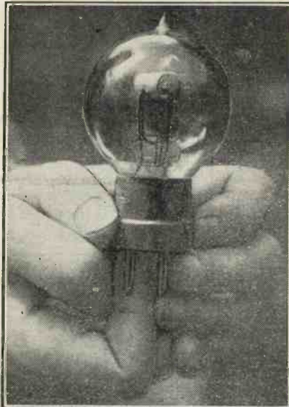
A bright-emitter valve that was "first-class" in its day. Note the "pip" on the bulb.
