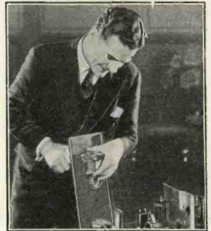
Mounting one of the variable condensers on the panel.
