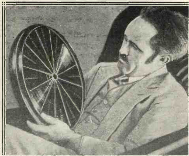
Hans Vogt, the German radio engineer and physicist, with his new capacity-type loud speaker—he calls it the Oscilloplan. It is said to give very promising results
