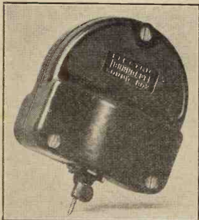
The Burndept "electrical sound-box." A good low-priced pick-up.
