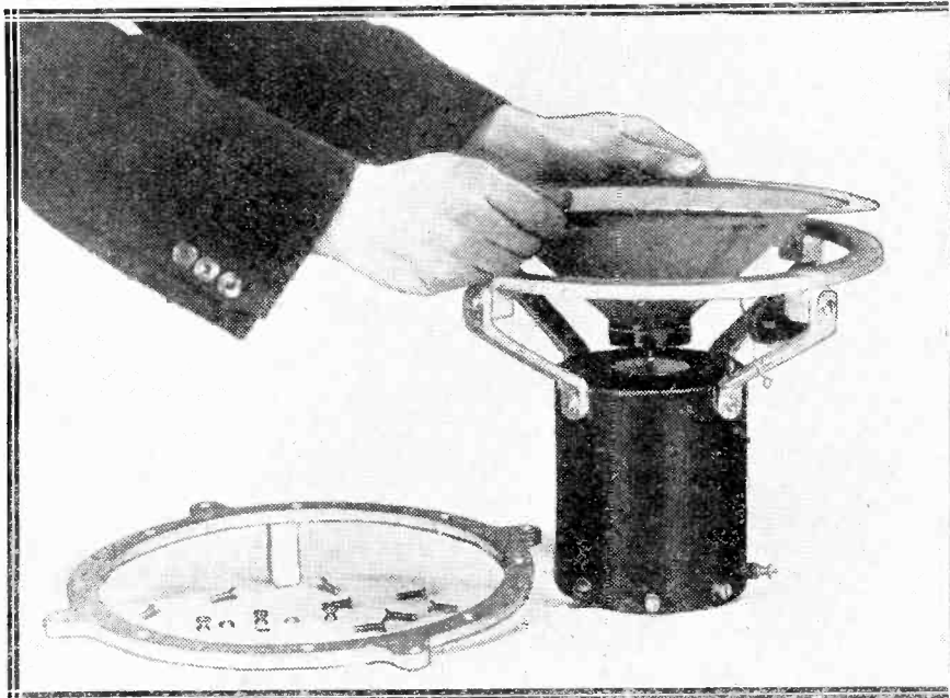
Dropping the completed diaphragm into position. The centre-maintaining device is only fitted when the unit is completely assembled. Holes in the cardboard ring are made when the moving coil is approximately centred in the annular gap.
