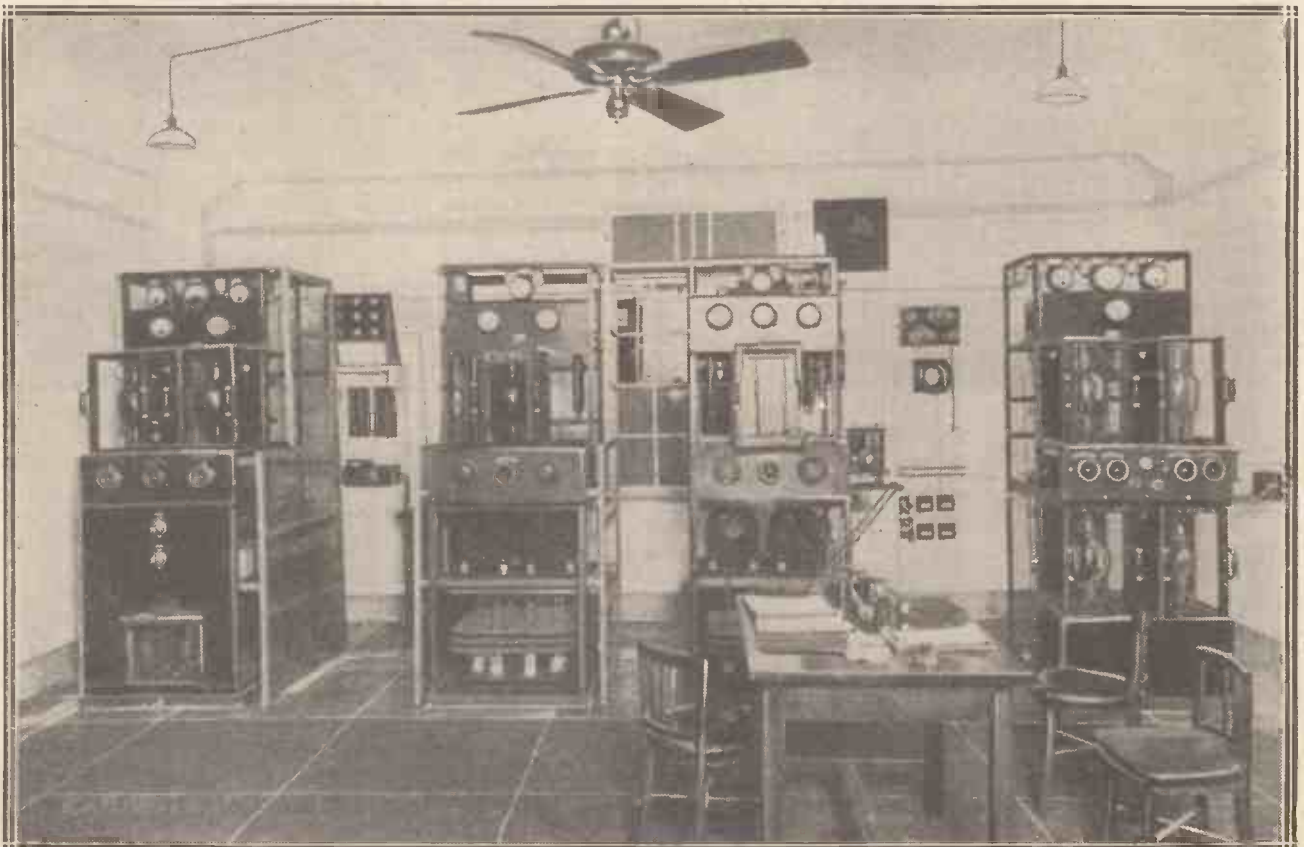
Though their programmes may not be of a very high order, and may be even more "talky" than our own, the Japanese follow Western methods in the design of their transmitters. This photograph shows the Nagoya transmitter, which is of the famous "Q" type and has a power of 6 kw.
