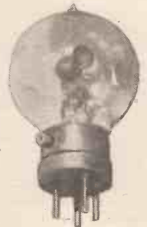
A four - electrode valve ; the connection to its additional grid is taken from the small screw terminal mounted on the side of its base.
