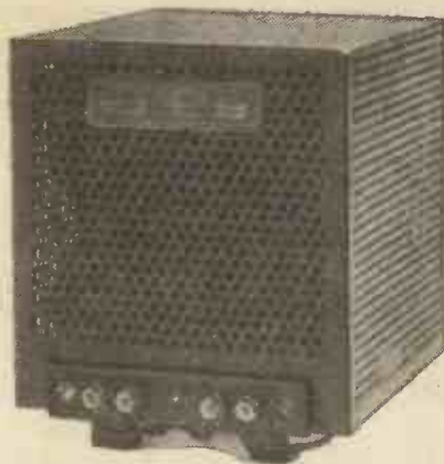
A typical Westinghouse rectifier set. The input is 110 volts at 50 cycles, output being 60-75 volts D.C. and 1.5 amp.
