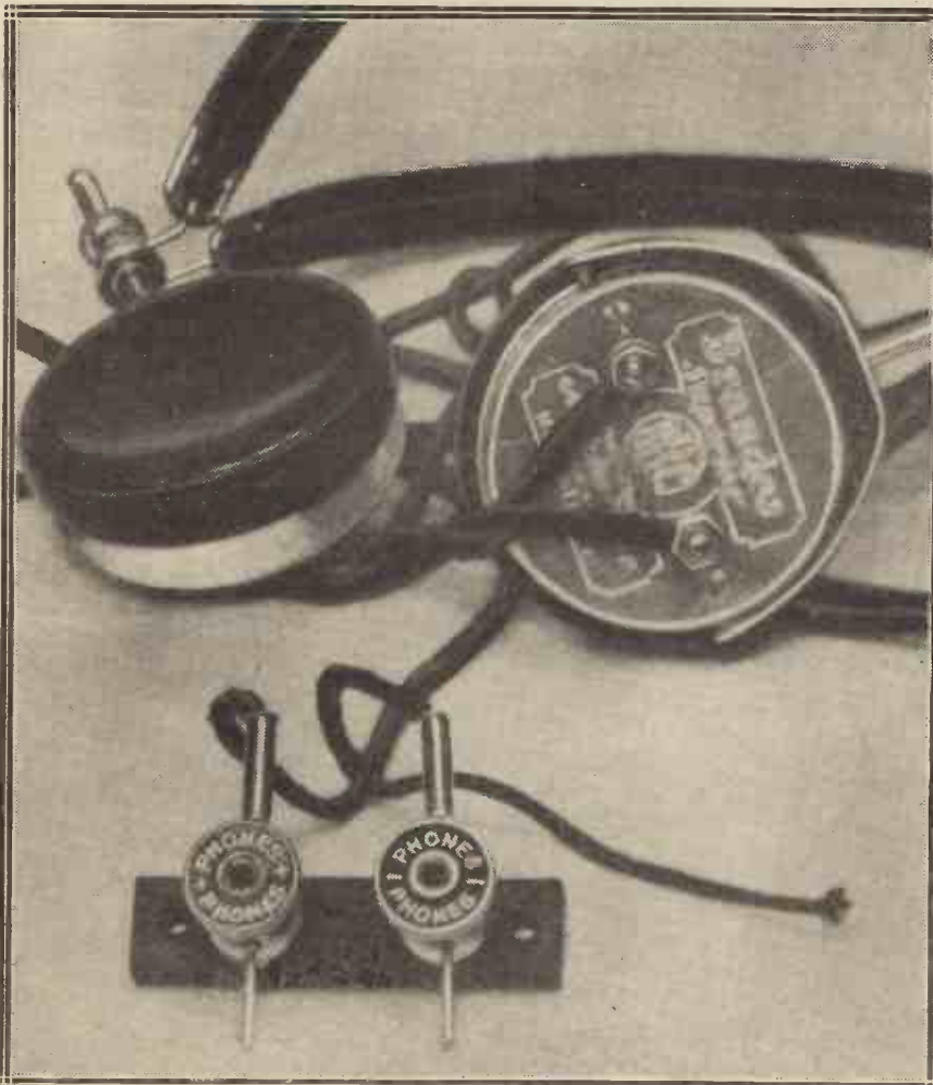
A simple telephone terminal board for wall mounting.
