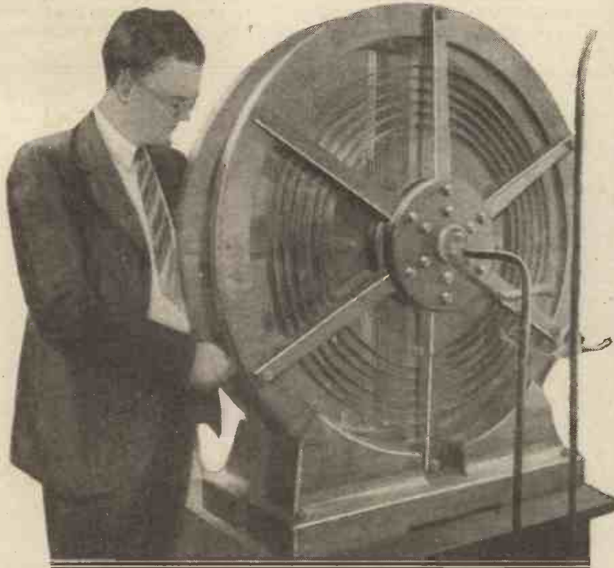
This is the aerial tuning coil used in connection with the new 50-kw. broadcasting plant at W E A F, Bellmore, L.I., N.Y. It is not unlike, in appearance at least, some of those plug-in coils used in short-wave receivers, and it serves a similar purpose. But there is a slight discrepancy in the similarity when it comes to a question of sizes.
