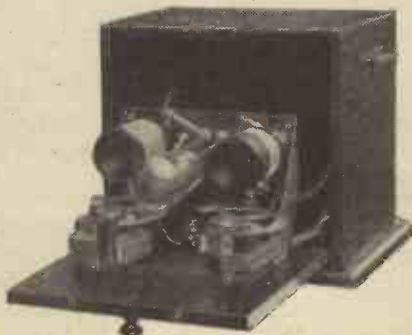
. . . here is shown how the front panel can be pulled forwards and downwards to reveal the interior of the set.
