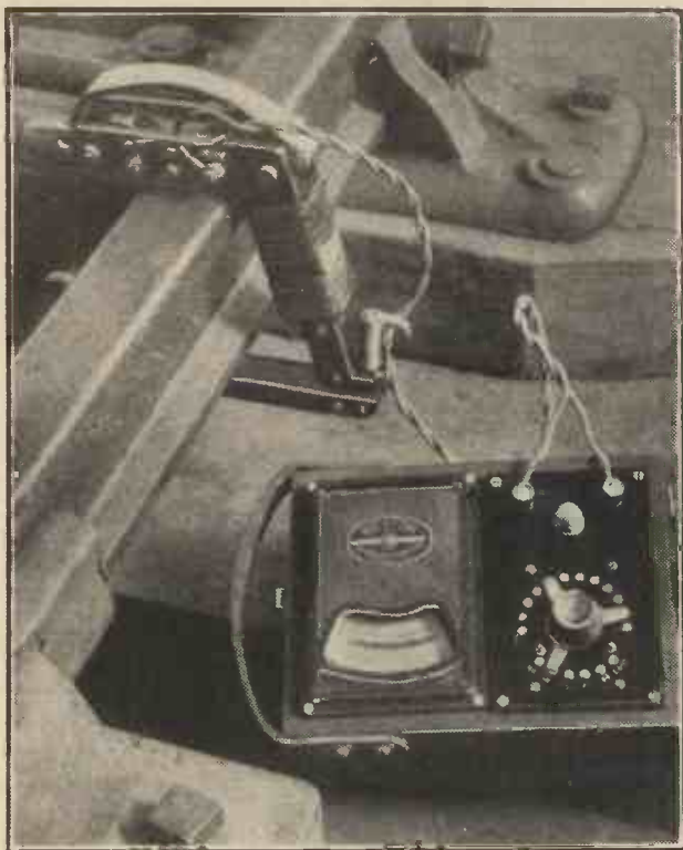
A new metal rectifier, of the type now being applied to wireless reception, is here shown embodied in a sensitive meter applied to railway signalling. Such is its efficiency that it can detect and register minute alternating currents, even though the rail to which it is affixed is carrying, at the same time, the very heavy direct current required for electric locomotives.
