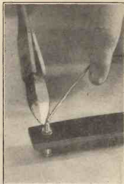
The soldering iron must touch both the terminal and the wire.
