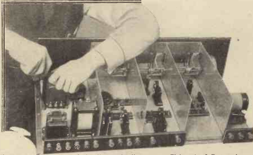
Nearing the completion of the "mounting" process. Fixing the L.F. transformer in position.
