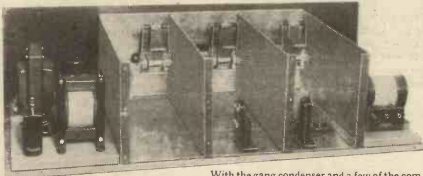
With the gang condenser and a few of the components mounted. Arranging preliminary layout details with experimental screens. The various sections of condenser are not coupled together.
