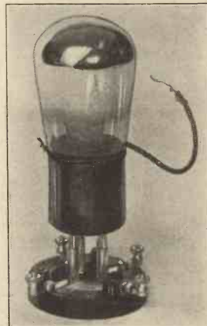
Robinson's new Interdyne valve fits the standard four-pin valve holder and is no larger than an ordinary receiving valve of average dimensions. The flexible lead that can be seen is the connection to the additional anode.
