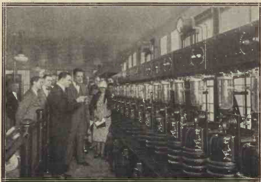
The transmitting valves used by the high-power American station, W E A F.
