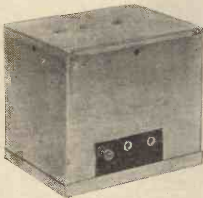
The wave-trap can be totally screened to prevent interaction with the receiver.
