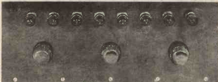
The knob on the extreme right controls the volume of the output, and the other controls give variations of voltage.
