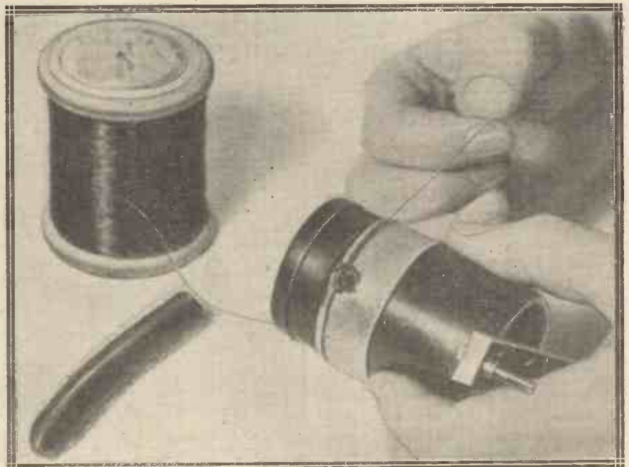
Another dab of Chatterton's keeps the primary in place during winding operations.
