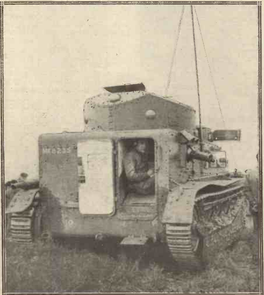
The wireless "cabin" on one of the latest "tanks." Note the aerial mast and the operator wearing phones.
