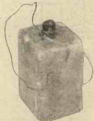
Fig. 5. Protecting the windings by means of wax.
