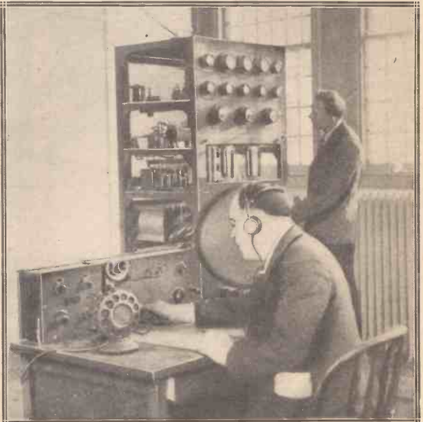
The transmitting room of the new New York broadcasting station WGL. This station is transmitting on a wave-length of 442 metres.
