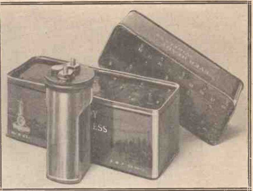
The H.T. and L.T. batteries employed in the original set.
