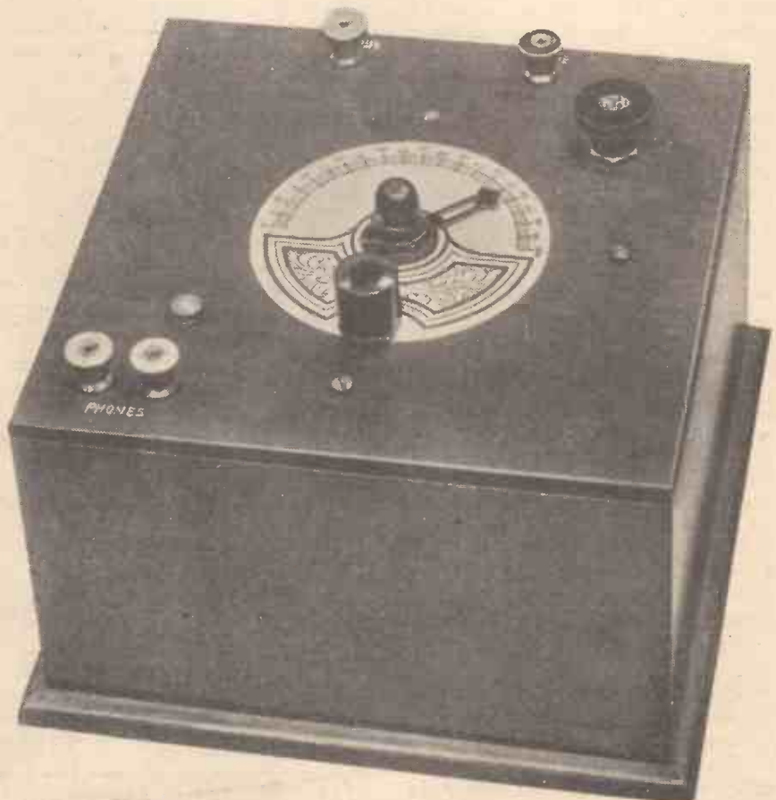
The use of a "fine-tuning" variable in a simple crystal set may appear to be rather incongruous, but it is really needed in this selective little "Ultra."
