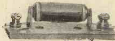
A crystal detector of the "permanent" type is recommended by Captain Round.
