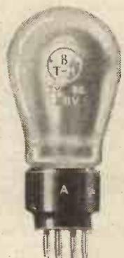
The New B8 resistance valve which is discussed in this page. For the last stage of amplification the B6 is advised by the makers.
