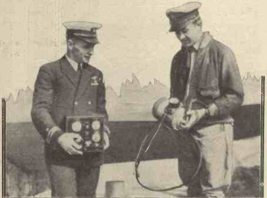
A “Nutshell” seaplane set. Evolved by the U.S. Navy, this set weighs only 8 lbs. It has a range of several thousand miles.
