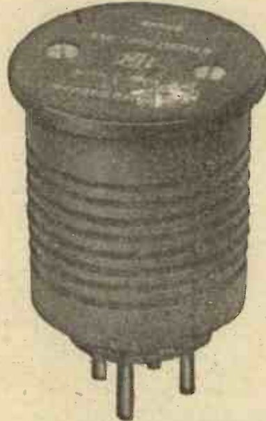
Fig. 3.—The original plug-in barrel type of H.F. transformer.
