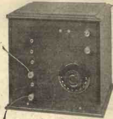
The two flexible connections are for aerial and earth.
