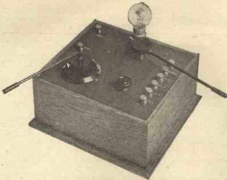
Successful tuning upon the wavelengths for which this receiver is designed can only be accomplished by the use of extension handles fitted to the condenser and reaction controls.
