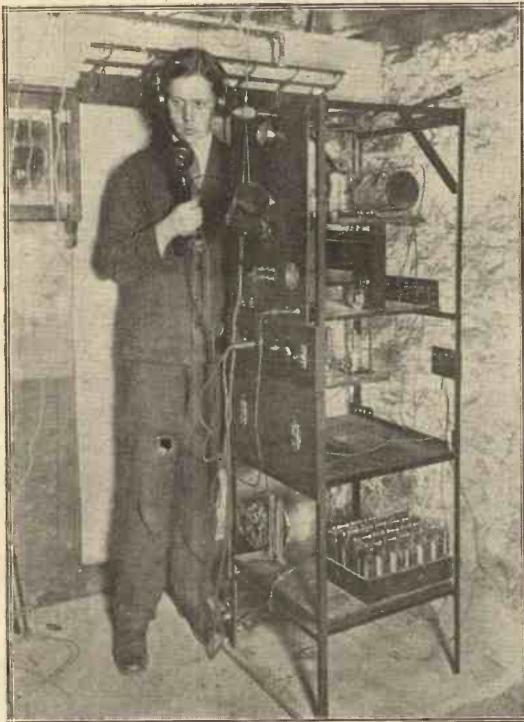
Many enthusiasts in America have miniature broadcasting stations of their own. The above photograph shows the 200 watt transmitter owned by Mr. E. W. Edwards, of Cincinnati.
