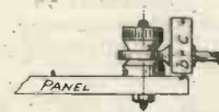
Fig. 2.—This diagram makes clear that the leads cannot be connected if reversed.
