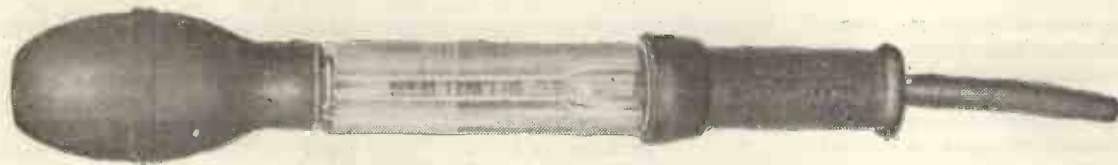
A typical hydrometer for testing accumulators
